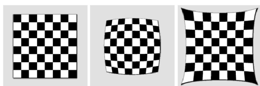
Fig. 1. Checkerboard images without distortion (left), with barrel distortion (center) and pincushion distortion (right).
