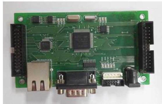
Fig. 5 The Developed Sub-Control Board for Industrial Communication Gateway
