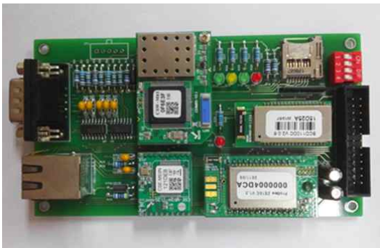
Fig. 6 The Developed Sub-Control Board for Industrial Communication Gateway
