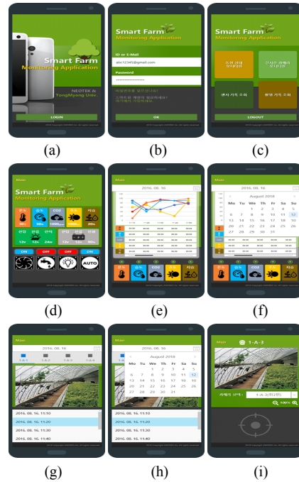
Fig. 7 Mobile-based remote detection system execution. (a) Smart Farm access main screen (b) Login screen (c) Mobile service main screen (d) Status monitoring configuration screen (e) Data display screen (f) Data inquiry screen (g) CCTV/Image inquiry screen (h) CCTV/Image data inquiry screen (i) CCTV control screen
