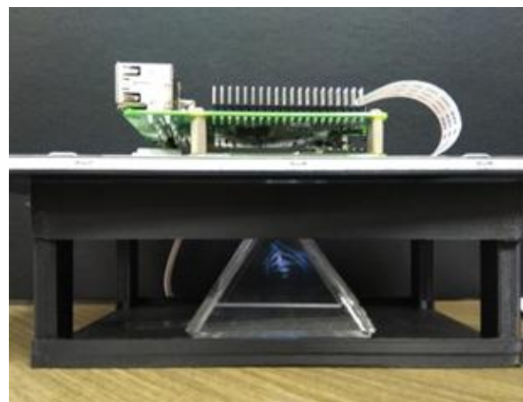
Fig. 7. Scaled model of hologram digital signage
