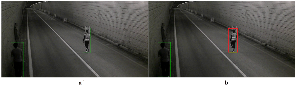
Fig. 2. bounding box overlapped tracking, a (the n th frame) and b (the (n+1) th frame)
