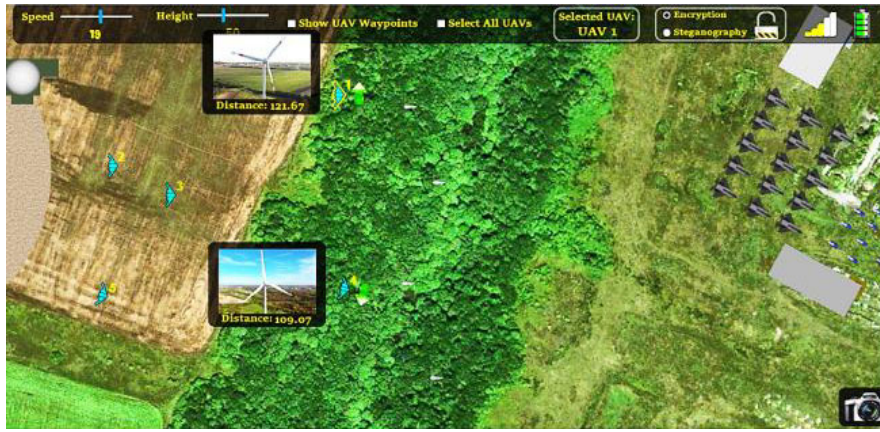
FIGURE 8 Overall view of the proposed intelligent adaptive interaction (IAI) for five unmanned aerial vehicles (UAVs). Selected UAV has been highlighted in yellow. Two simultaneously occurred collisions and their accordant temporal in-place UAV's camera displays at the back of the UAV's icons have been depicted
