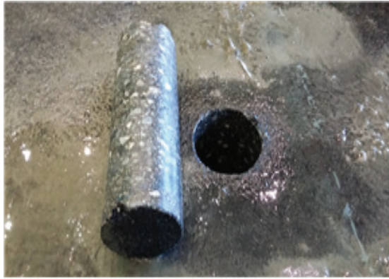
Fig. 3 Wet core specimens
