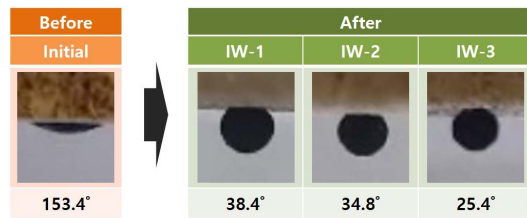
Fig. 7. Contact angle results showing wettability alteration after LSPF.
