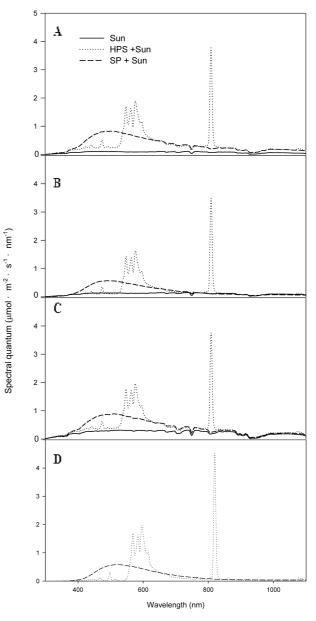
**Fig. 4.** Spectral quantum distributions with time in the greenhouses under sunlight with no supplemental lighting (Sun), sunlight with high-pressure sodium lamp (Sun + HPS), and sunlight with sulfur plasma lamp (Sun + SP): (A) before sunrise, (B) after sunset, (C) cloudy day, and (D) midnight on 2 March, 2016.
