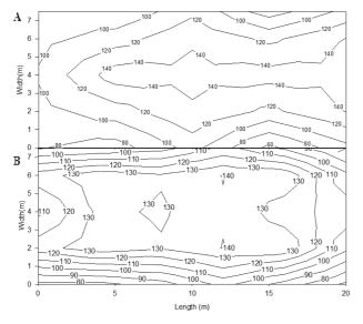
Fig. 2. Distributions of photosynthetic photon flux density  $(\mu mol \cdot m^2 \cdot s^{-1})$  at the floor of the greenhouses where high pressure sodium lamp (A) and sulfur plasma lamp (B) were installed.
