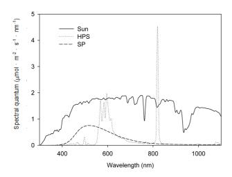
Fig. 3. Spectral quantum distributions of sunlight (Sun, 11:00 on 2 March, 2016), high-pressure sodium lamp (HPS), and sulfur plasma lamp (SP) used in the growth chamber.
