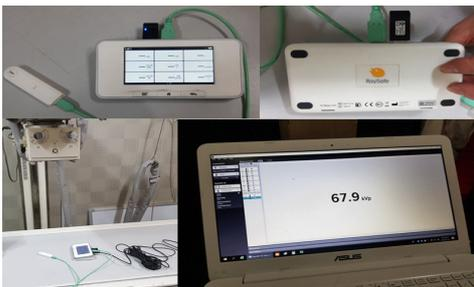
Fig. 4. X2 Base unit of Raysafe. (kVp meter)
