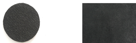
Fig. 3. Fabricated specimen for (left) radon and (right) HCHO/VOCs for reduction capability assessment.
