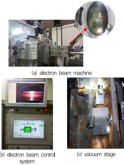
Fig. 3 Setting up devices for electron beam processing
