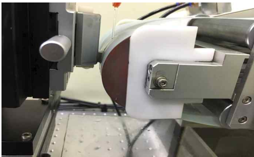
Fig. 7 Image of polishing process for SUS 304 specimen
