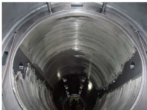
Fig. 4. After stern tube bearing damage.
