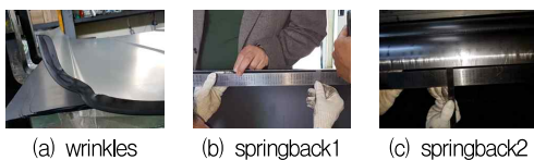
Fig. 2 Examination of problems in existing forming process
