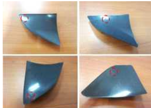
Fig. 10 Products using fluid cooling
