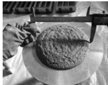
**Photo 2** View of flow test
