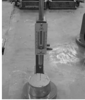
Photo 3 View of air contents test Photo 4 View of vicat Test
