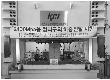
Fig. 8 Load Transfer Test (30,000 kN)
