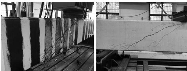
(a) CFRP strip fracture (b) shear failure
