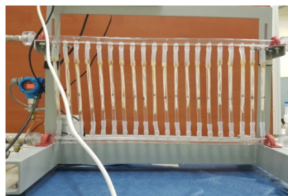
(b) Accelerated ageing apparatus
