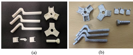
Fig. 11. 3D printed parts (a) ABS polymer (b) Stainless steel (STS 316L)
