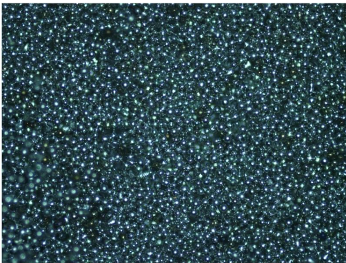
Fig. 3. Microscopic photo of stainless steel powder (AM 316L cE) with the diameter size of more than 32 \mu\text{m}
