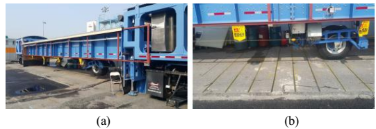
Fig. 9. Experimentation of wheel load (a) View of the APT (b) Application of wheel load
