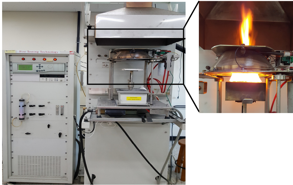
Figure 2. The photograph of cone calorimeter equipment.
