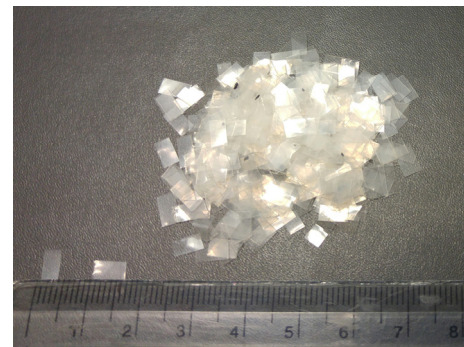
Fig. 2. Vinyl strips used in the study (3mm×6mm)
