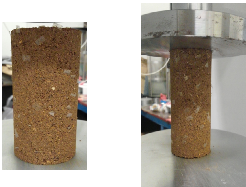
Fig. 3. Molded specimen (50mm×100mm)
