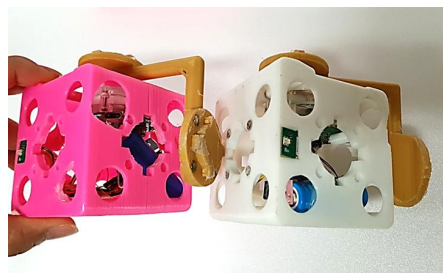
Fig. 3. Docking process of two modular blocks
