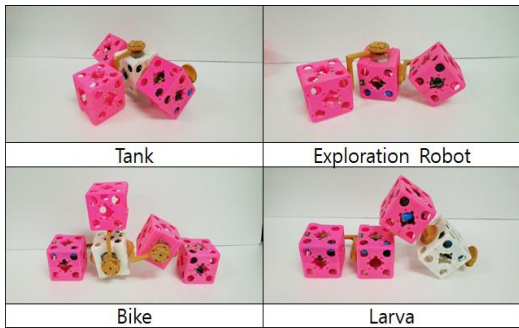
Fig. 4. Combination examples of modular robot
