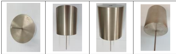
Fig. 2. Penetration steel wire and drop weight
