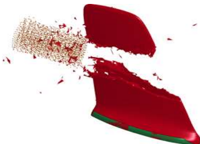
Fig. 4 Steady Flow Shape of Bird Strike(excluding Foam)
