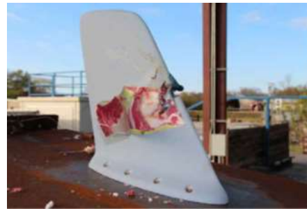
Fig. 10 Dummy Antenna Test Result
