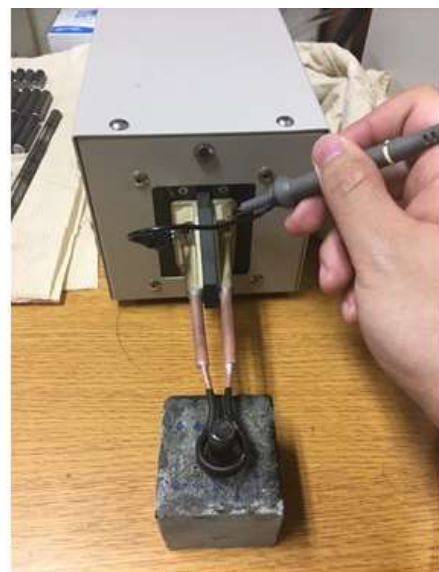
Fig. 1 Configuration of induction heating device
