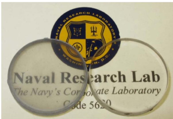
Fig. 11. Transparent \text{MgAl}_2\text{O}_4 ceramics made from commercial powder(left) and acid-purified powder(right), Reproduced with permission from Ref., 135) Copyright 2015, OSA publishing.
