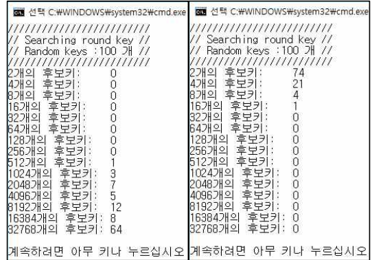
Fig. 6 The number of round key candidates using one or six correct-faulty cipher text pair(s)
