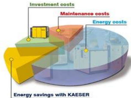
<Figure 4> Costs related to air compressor installation and maintenance
