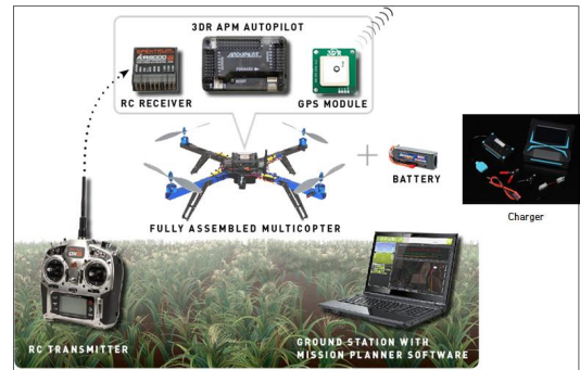
Fig. 1. Introducing Copter(The general structure of the Drones) [8]
