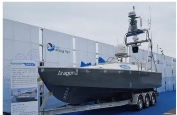
Fig. 1 Aragon II, Unmanned surface vehicle of KRISO
