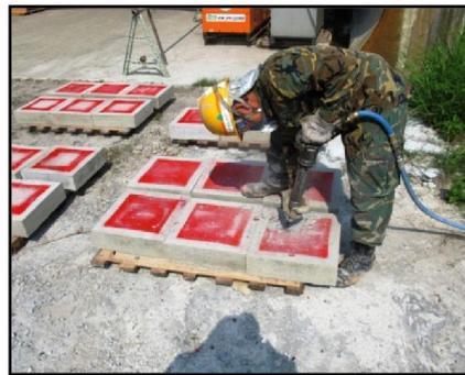
**Fig. 3.** View of chipping by hand-held breaker.
