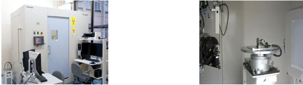
Fig. 1. Micro focus X-ray CT scanner at kumamoto university.
