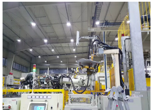
〈Figure 9〉 Sealer Vision Inspection Equipment Installed on NEOTEC Factory Production Line
