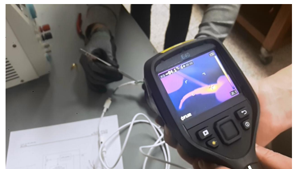
[Figure 11] Measurement of Temperature Rise
