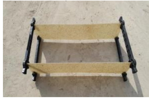
(b) Assembly of GFRP plate
