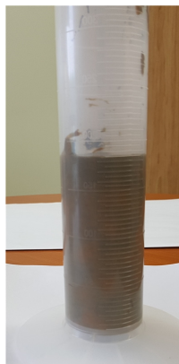
(a) Sequential mixing of water, cement and bentonite for 20 minutes
