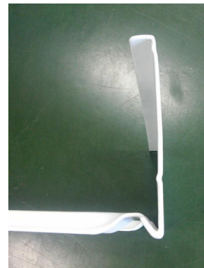
Fig. 10 Cable tray after roll forming process
