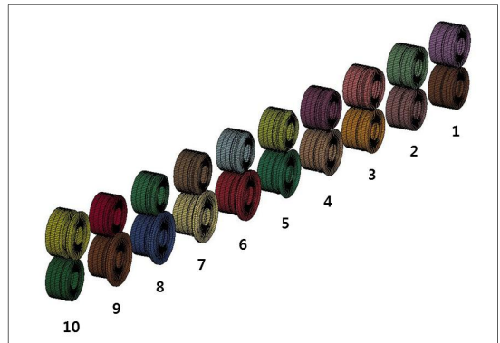
Fig. 5 (a) Roll design from 1 st to 10 th stands
