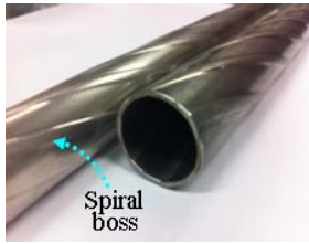
Fig. 8 Actual scene of spiral-boss tube drawn from rotational die with rotation insert
