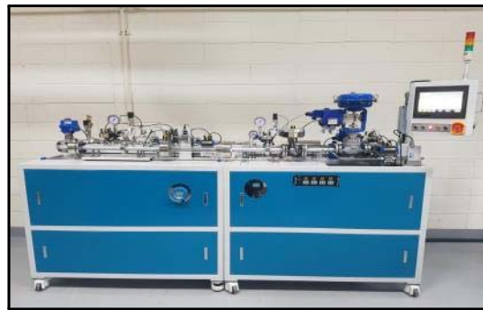
Fig. 13. EFV performance test facility installed in KGS
