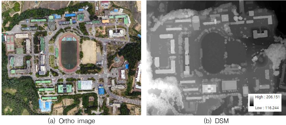
FIGURE 14. Production of UAV photogrammetry using UAV image
