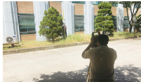
FIGURE 12. Tree height observation using total station
