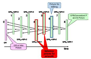
Fig. 1. Presentation of low-delay coding structure.
