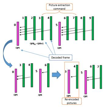
Fig. 3. Example of decoding and re-encoding procedure during the picture extraction.
