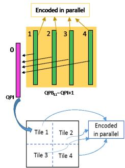
Fig. 4. Picture and tile level parallel processing.
