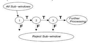
Fig. 5. Cascade process in Haar cascade method.
