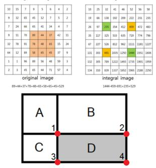
Fig. 3. Integral method of Haar cascade method.
