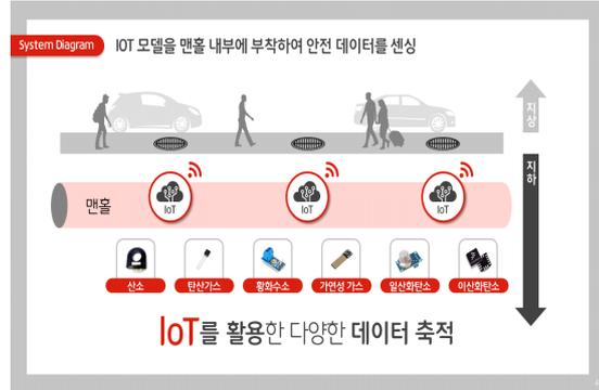
Fig. 2 Monitoring of harmful gas using LoRa network
