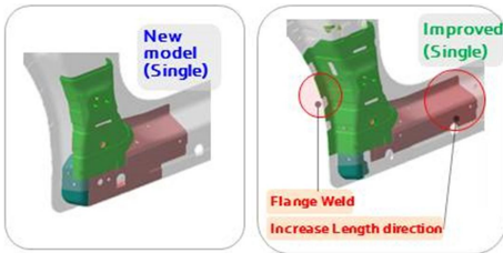
Fig. 14 A Pillar Lwr Concept (“ㄷ”, “ㄱ” Section)
