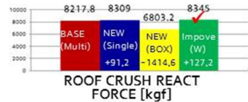
Fig. 18 B Pillar Case analysis data of Roof Crush
