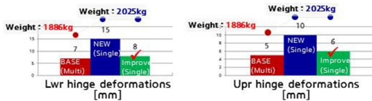
Fig. 15 A Pillar Lwr Hinge Deformations of Smalloverlap test
