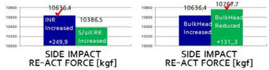
Fig. 23 Case Analysis of B Pillar LWR Structure type of Side impact
