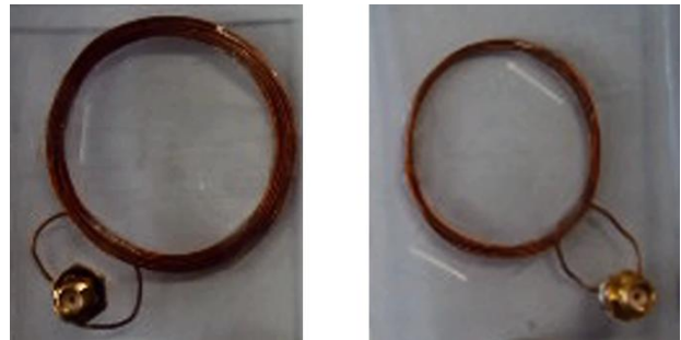
Fig. 8. 6 turns and 3 turns with the diameter of 37~46mm.
