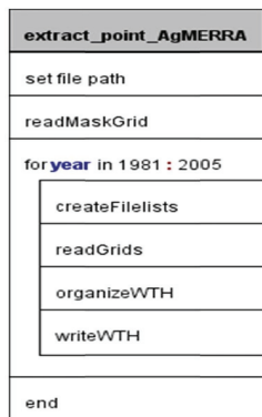
Fig. 1. The Nassi-schneiderman chart for extract_point_AgMERRA.R to prepare weather input files for the AgMERRA data files that have a gridded data format.
