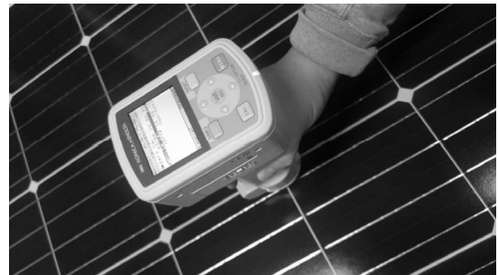
Fig. 1. Implementation of YI (Yellowness Index) equipment
